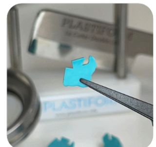
Example of use of the P25 for dimensional control
