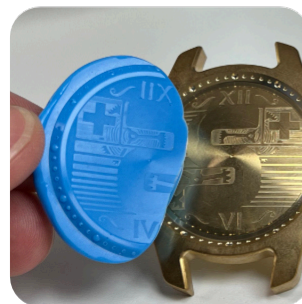
Example of use of the P80 Ra for roughness control
