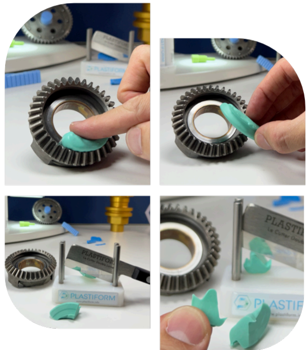
Example of use of the M25 for profile control
